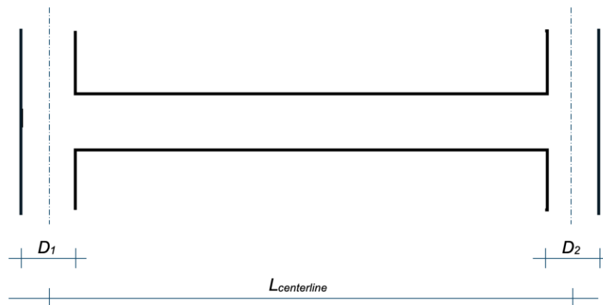
FIG. 4 GEOMETRY OF A MEMBER MEETING OTHER MEMBERS AT ITS ENDS
